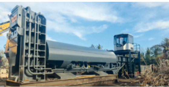
KOLOSS 1000, 8-meter box, force of the lids: 400 tons each, 600 HP diesel engine (electric version available)
